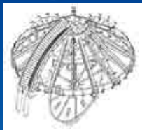
MERIDIAN WELDING & MACHINING FIXTURE FOR TANK DOMES OF PSLV & GSLV STAGE 2
