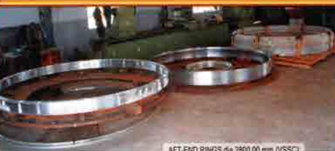
AFT-END RINGS dia 2800.00 mm (VSSC)
