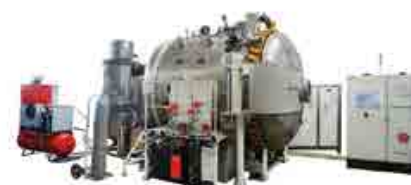
Cabin Environment Simulation System to Carryout Functional Evaluation of Space Oriented Modules
